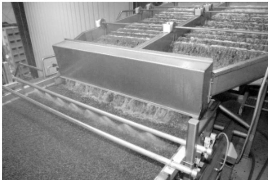
**Above:** Raisins cascade through the washing process, which yields between 60,000 and 80,000 gallons per day of wastewater. **Below:** Fresh from the washing cycle, raisins are sprayed with clean water.
