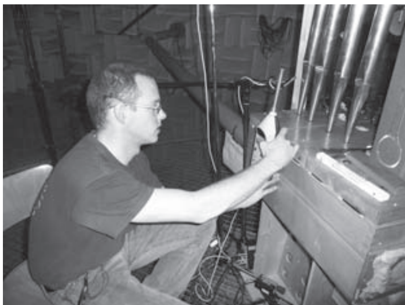
Measuring sound pressure levels on the test pipes
