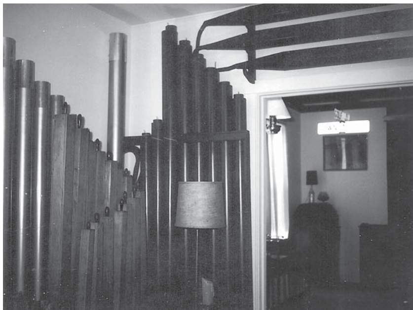
Even with a 9-foot ceiling, pipes of the 16' Haskell Violone were mounted horizontally, and a few of the 16' Bourdon were laid on the floor.
