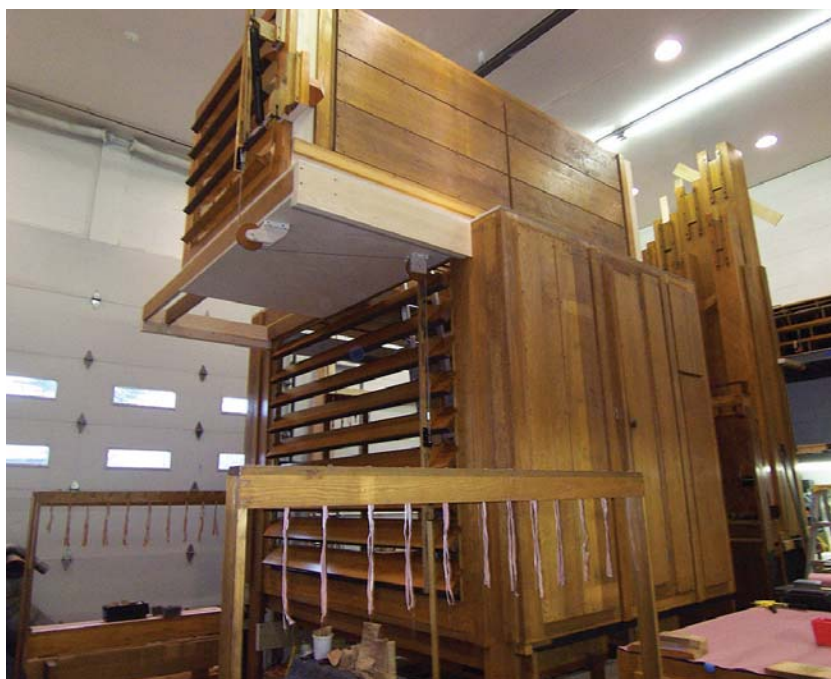
The Choir/Great/Pedal chamber during erection at FBI's Tolland, Connecticut facility. Special elevated chamber houses the harp.
