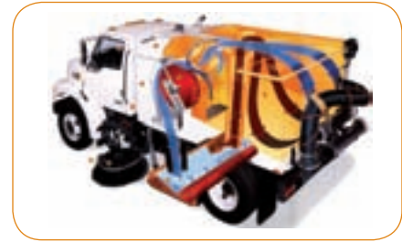
The inner workings of a regenerative air sweeper.
