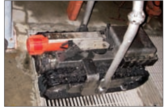
Responder robot inspections reduced Palo Alto's scope of sewer work by nearly one half.
