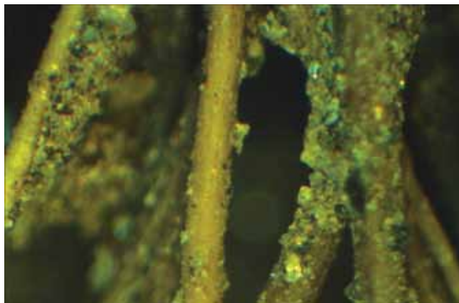
Used fiber filter coated with particles
