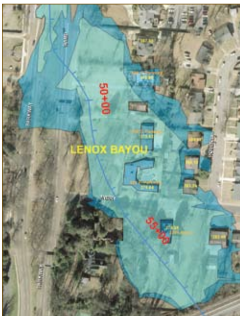
Figure 1. This preconstruction flood map illustrates the current impact of both a two-year (in green) and a 100-year (in blue) storm.
