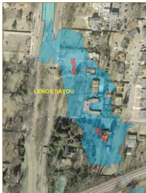
Figure 2. This postconstruction flood map shows the area that a 100-year storm would flood; no flooding is expected with a two-year storm.
