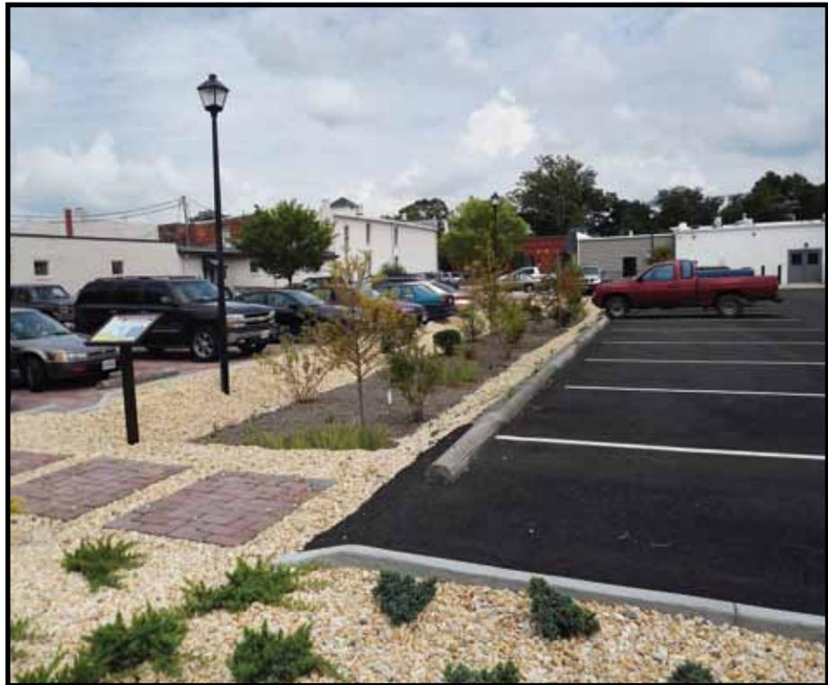
an economical solution to costly storm water planning and regulation. The system uses dollars already budgeted for an impervious wearing surface and converts them into part of the storm water management plan, replacing the impervious asphalt or concrete with a permeable paver section.
