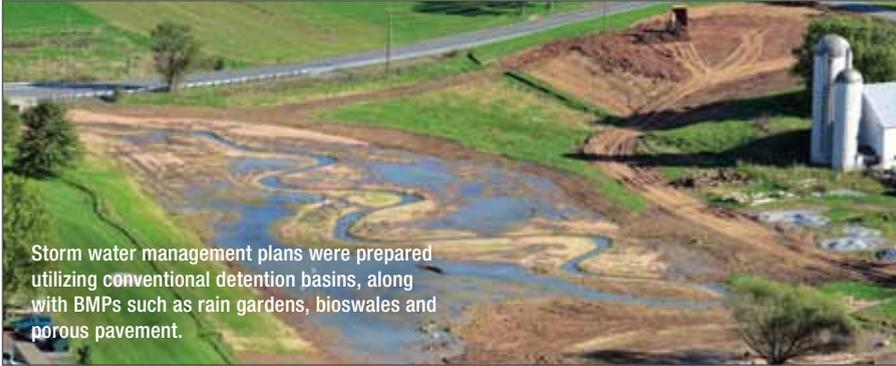
Storm water management plans were prepared utilizing conventional detention basins, along with BMPs such as rain gardens, bioswales and porous pavement.
