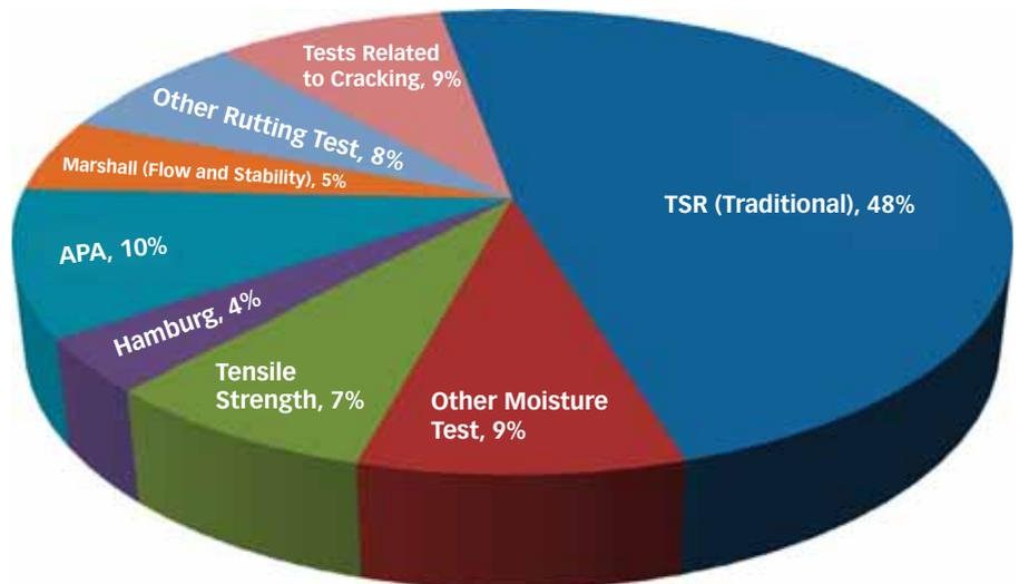
**Figure 2. Breakdown of the performance testing requirements by DOTs.**
