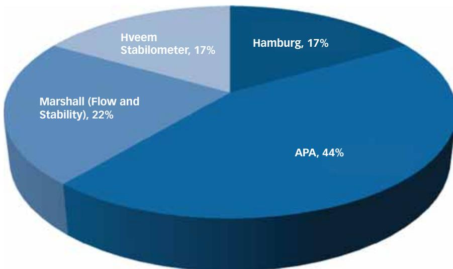
**Figure 4. Cracking performance tests used by DOTs.**
