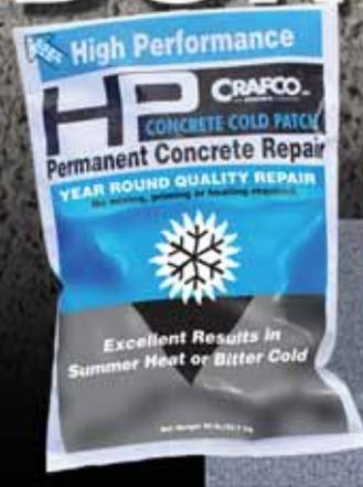
Unlike most other concrete patching materials, HP Concrete Cold Patch requires no heating or special installation equipment. HP Concrete Cold Patch will repair potholes, spalls or any other confined voids in concrete that are greater than 1/2 inch deep and 1 inch wide. HP Concrete Cold Patch is EASY, FAST and PERMANENT.
