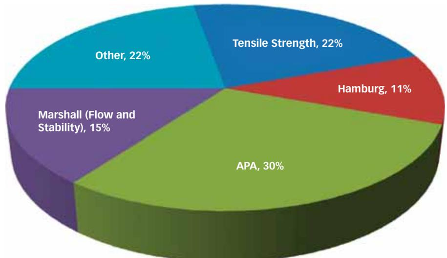
**Figure 3. Rutting performance tests used by DOTs.**
